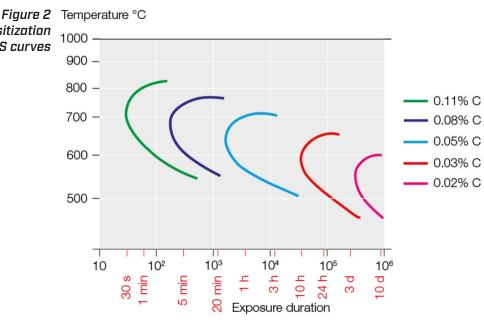
Limitations The temperature range below 450 - 700°C should be avoided, as it may lead to sensitization of the microstructure of this steel through the formation of intergranular precipitates, which weaken it and reduce its corrosion resistance. In this case, a solution annealing treatment at 1040-1080°C is recommended.
